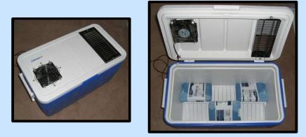
Keeping the floor vent closed and a piece of cardboard taped over the fan motor will help keep the ice from melting until you are ready to use the portable A/C unit.
